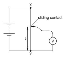
He changes the length of wire l by moving the sliding contact along the resistance wire.
